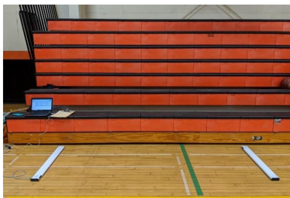
Figure 2. Set-up for testing reactive strength index using the MuscleLab Ergotest infrared contact grid.
